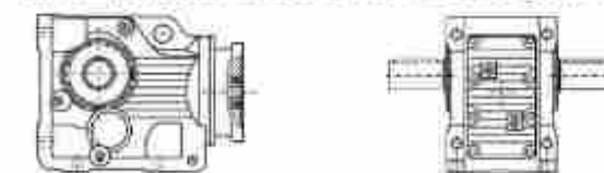
KA (K, KF, KAF, KAB, KAZ) ...Y... 电机用户自配或配特殊电机时需加取接法兰 When equipping the user's motor or the special one, the flange is required to be connected
